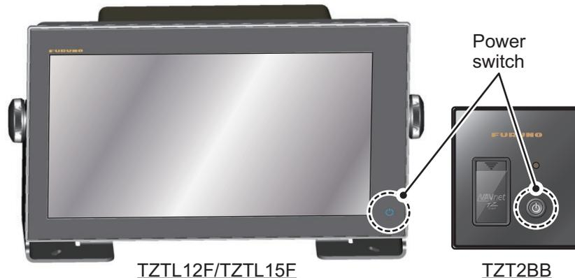
When you turn on the power, the equipment beeps twice and the start-up screen appears. After the startup process is completed, the [NAVIGATION WARNING] screen appears. Read the warning, then tap [OK]. Then, the last-used display appears.
