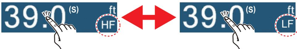
**Method 2:** Tap the screen to show the pop-up menu. Tap [Frequency], then tap the flipswitch of [HF] or [LF] as appropriate.
