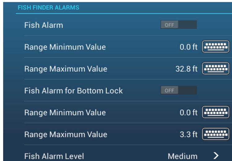
3. Set the start depth in [Range Minimum Value], the end depth in [Range Maximum Value].
